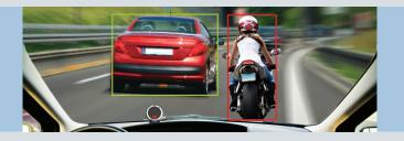
etc. The system measures the distance from the vehicle's wheels to the lane markings on both sides. Studies conducted on Fleets showed a 65% decrease in all lane-departure related crashes using vision-based LDW systems.
